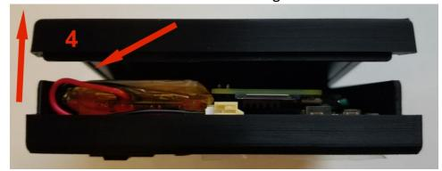
4. That's it! The other side should slip right out, exposing the device internals.
